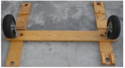
Rails and crossbar laid out but not assembled and crossbar not positioned in slots so you can see how the crossbar will fit into rail slots
